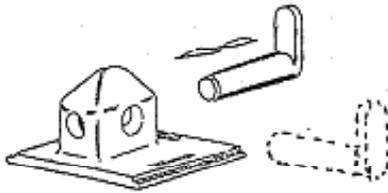
SISTEMA "C" ESQUINERO CON PIN DE SEGURIDAD (I.S.O 3874)
