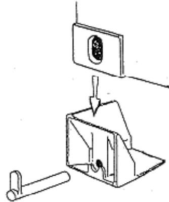
SISTEMA "D" TRABA DE BISAGRA LATERAL CON PIN DE SEGURIDAD (PARA VAGON ADAPTABLE A CAMION)
